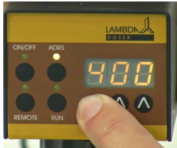
Figure 2-4: Set the desired flow rate value for the first program step by pressing the buttons ▲▲▲ below the display (from 0 to 999, corresponding to 0 to 100% of the motor rotation speed).
