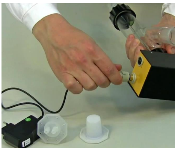
Figure 1-11: The 12 V connector of the power supply is plugged into the 12 V DC socket of the motor unit and the power supply is connected to the mains.
