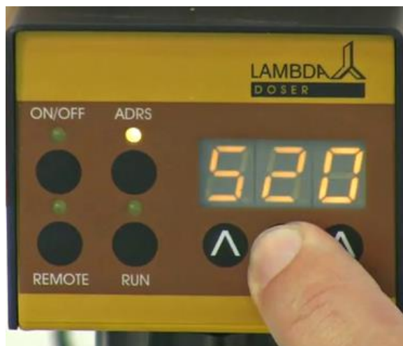
Figure 2-8: You can now enter the desired flow rate for the second program step.
