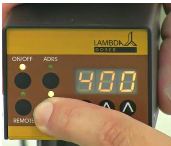
Figure 2-16: To START the program, press the RUN button. The RUN and ON/OFF LEDs are on.
