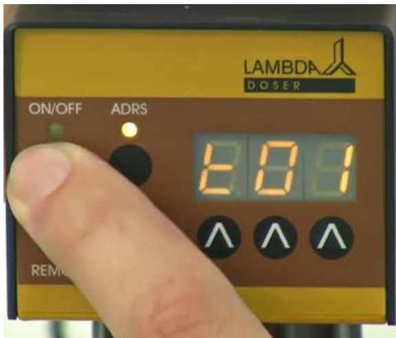
Figure 2-5: Press the ON/OFF button. The indication "t01" will appear for a few seconds on the display indicating that you can program the time period of the first step in minutes or 0.1 minute steps.
