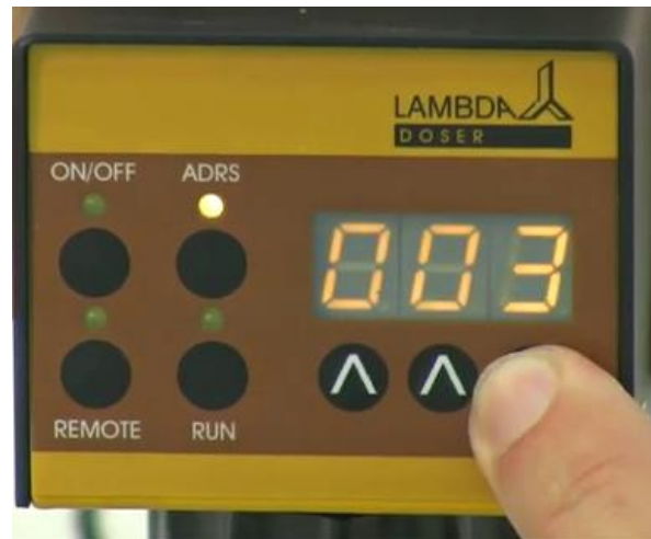
Figure 2-6: Select the desired time period for the first program step by pressing the buttons ▲▲ below the display (from 0 to 999 minutes or 00.0 to 99.9 minutes). By pressing the ADRS button, the time resolution can be set in minutes or 0.1 minutes. In the 0.1 minute time resolution a dot is displayed, e.g. "00.1".
