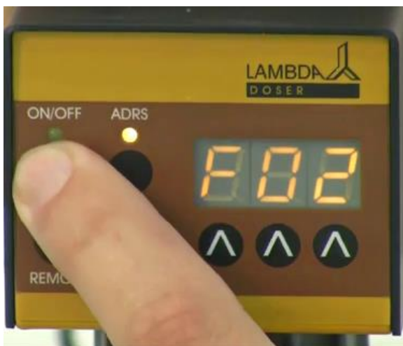
Figure 2-7: Press the ON/OFF button. The indication "F02" will briefly appear on the display.
