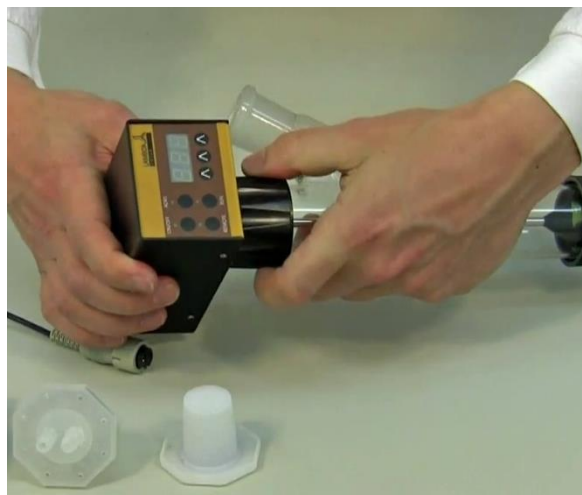
Figure 1-10: Press the axis of the motor unit completely inside the centering part. So that the metal pin of the motor unit will fit into one of the six corresponding holes in the centering unit. This assures a perfect seal of the DOSER and a sufficient pressure of the distributor against the Teflon disc in the bottom of the Doser vessel.
