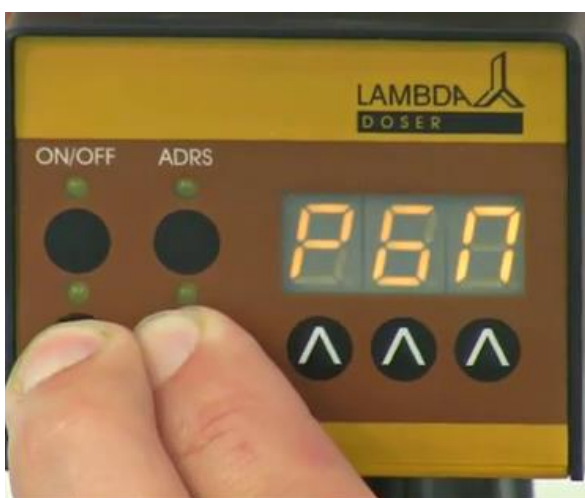
Figure 2-1: Pressing Remote and Run buttons simultaneously and the “ PGM ” indication appears.
