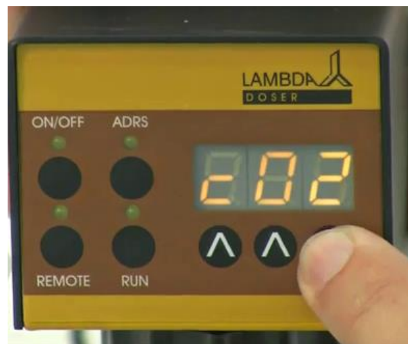
Figure 2-14: If you wish to repeat the same program 2 times, increase the cycle number to “c02” by pressing the buttons \wedge \wedge \wedge below the display (from 0 to 99 cycles). The program can be repeated up to 99 times, indicated by “c99”. If 0 is entered for the cycle number “c00”, the program will run continuously ( infinite loop ).
