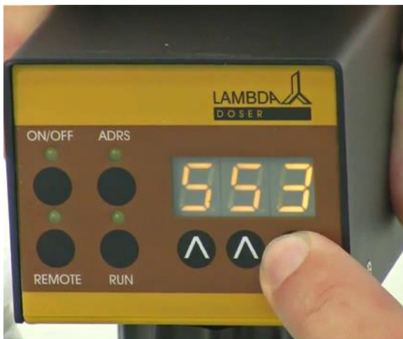
Figure 1-13: Choosing the speed of powder addition with the help of control buttons ^ ^ ^ .
